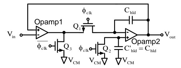
Modern SC sampling circuit for signal-independent sampling in IC
