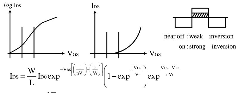
where  $V_t = \frac{kT}{q}$  and  $V_{Th}$  is threshold voltage
